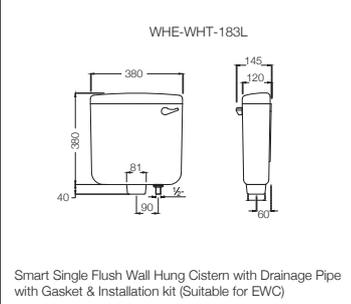
Smart Single Flush Wall Hung Cistern with Drainage Pipe with Gasket & Installation kit (Suitable for EWC)
